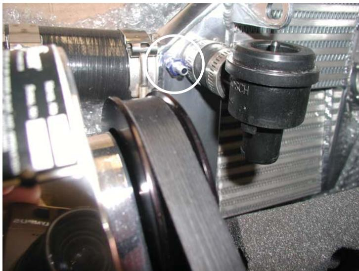
Boost Signal Amplifier (Front Mount Intercooler)
