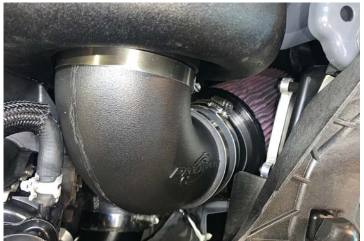
Plastic Inlet Installed
