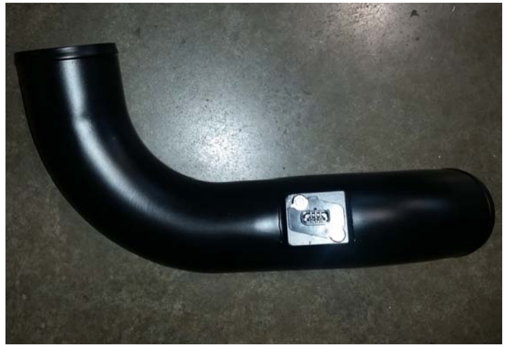
MAF Installed Into Tube #430
