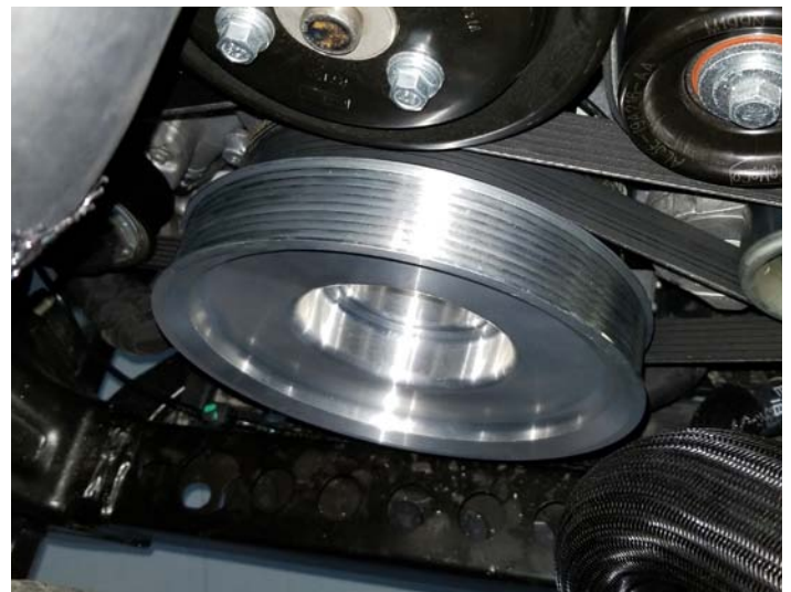
Crank Pulley Installed
