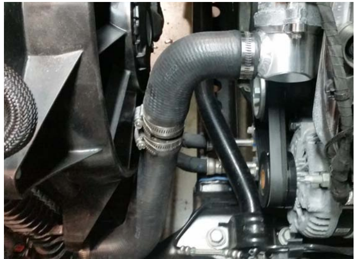
Upper Hose Section Installed
