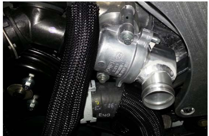
New Thermostat Housing Neck Installed
