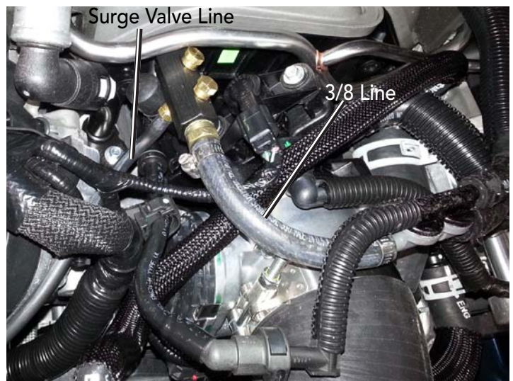
Vacuum Manifold Installed
