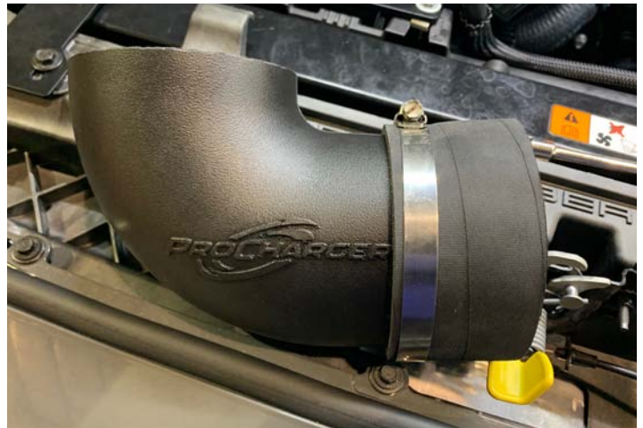
Plastic Inlet Installed
