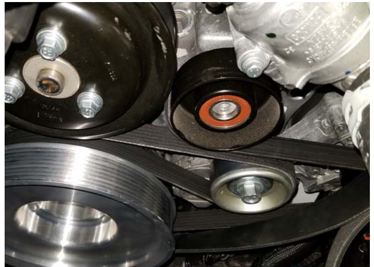
New Idler Shaft Installed
