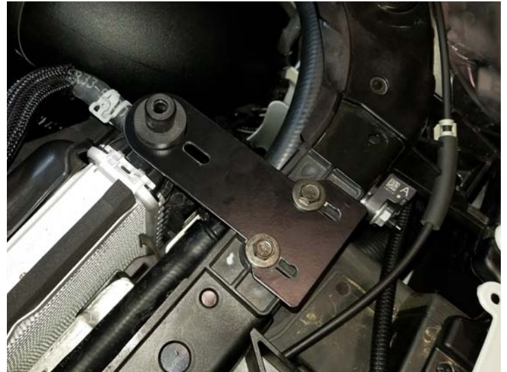
Radiator Bracket Installed
