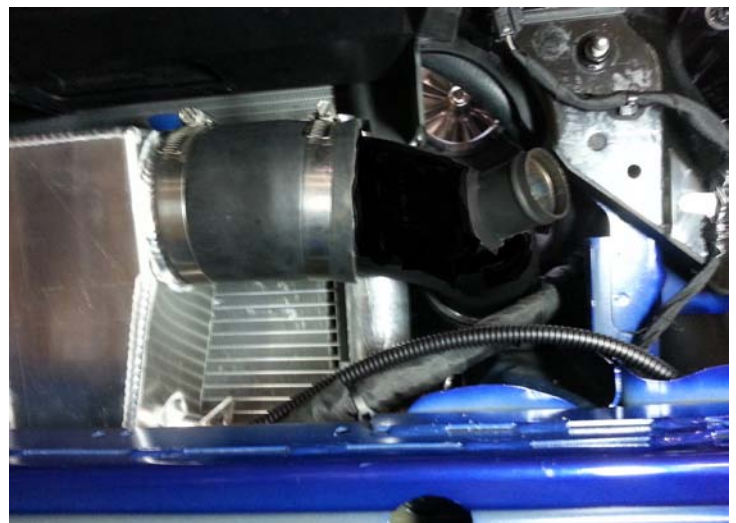
Surge Tube #380 Installed
